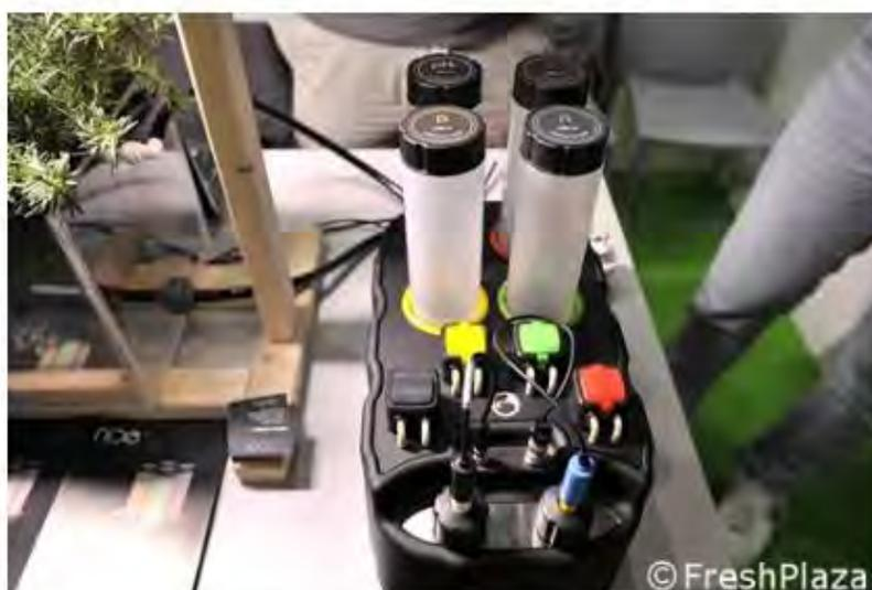
"Our automated management system - explains Andrea Carloni - can be installed in a few minutes. Two holes in the nutrient solution tank are enough to make the greenhouse automated and connected. It is compatible with any existing hydroponic system. It is ideal for any above-ground solution, up to 2500 liters of plant nutrient solution".
